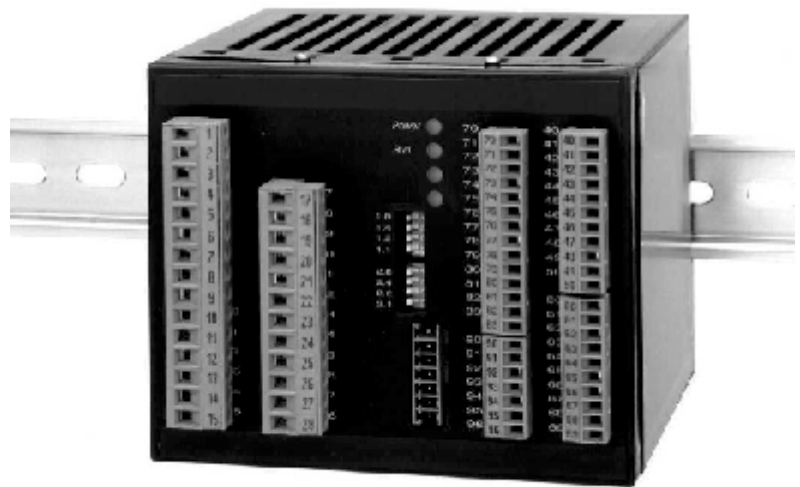
R 2200: 4-, 6-, or 8-zones temperature controller DIN-rail mounting. 35mm DIN-EN 50022
