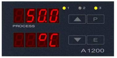
Format: 96x48 mm (1/8-DIN) Installation depth: 122 mm
