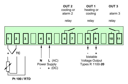
It is not permitted to connect the grounds of the sensor- and bistable voltage outputs with each other.
