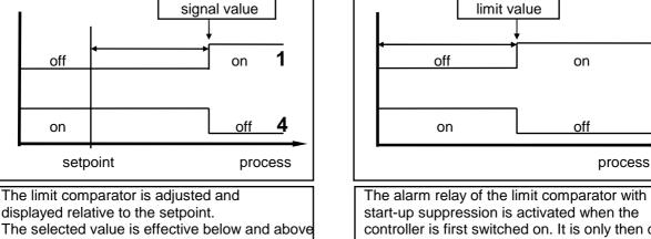
displayed relative to the setpoint. The selected value is effective below and above the setpoint. Switching behaviour: **Configuration:** limit range 3 off on 6 on off on setpoint process
