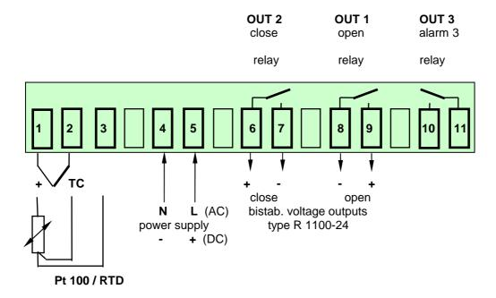
It is not permitted to connect the grounds of the sensor- and bistable voltage outputs with each other.
