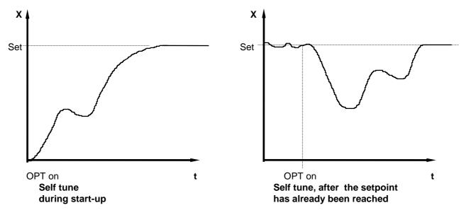
Self-tuning can be stopped by selecting the option OPT = OFF and pressing the "E" - key.
