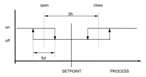
3-point-stepping controllers use PI control action in combination with motor actuators. It is important, that Sh should be several times larger than Sd. Switching frequency is dependant on the pre-selected feedback values.
