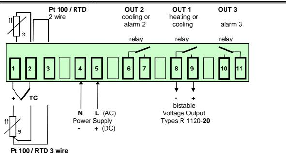
It is not permitted to connect the grounds of the sensor- and bistable voltage outputs with each other.
