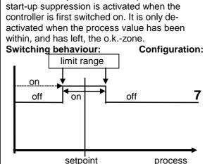
on: Relay "activated" off: Relay "not active"
