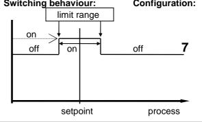
on: Relay "activated" or bistable voltage output "high". off: Relay "not active" or bistable voltage output "low".
