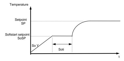
During the softstart the controllers' output response is limited to a pre-selected ratio, in order to achieve a slow baking out of high performance heat cartridges. Simultaneously the output clock frequency is quadrupled. Once the process value reaches the softstart setpoint, it remains stable at this value for a pre-selected hold-duration time. At the end of this period the process value rises to the valid setpoint. This results in a slower, more regular heating period.
