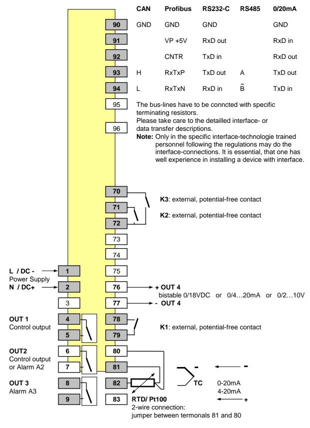
It is not permitted to connect the grounds of the sensor- and bist. voltage-outputs with each other.
