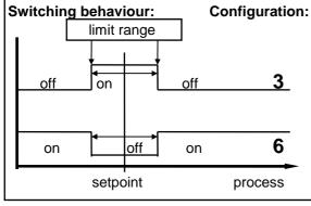
The alarm relay of the limit comparator with start-up suppression is activated when the controller is first switched on. It is only then deactivated, when the process value has been within, and left, the o.k.-zone.
