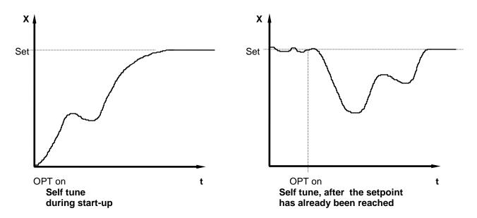
Self-tuning can be stopped by selecting the option OPT = OFF and pressing the "E" - key.
