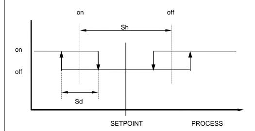
3-point-step-controllers use PI control action in combination with motor actuators. It is important, that SH should be several times larger than Sd. Switching frequency is dependant on the pre-selected feedback values.
