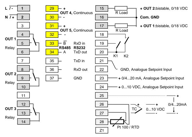
It is not permitted to connect the grounds of the sensor-, bist. voltage- and continuous-outputs with each other
