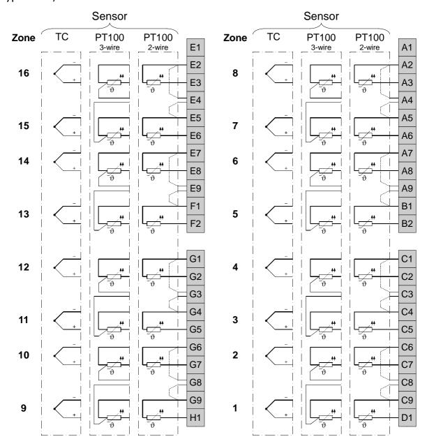
It is not permitted to connect the grounds of the sensor-inputs and Logic-outputs with each other.
