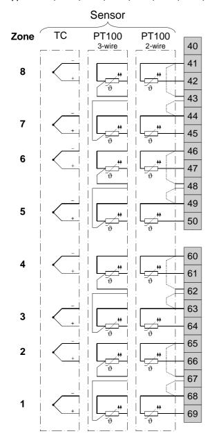
It is not permitted to connect the grounds of the sensor-inputs and Logic-outputs with each other.
