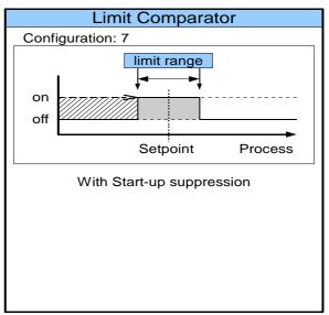
Each alarm contact works as a common alarm for all zones. The individual alarms A1 (A2) of all zones are connected to the common contact A1 (A2). The selected configuration is valid for all active zones
