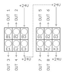
The power supply for the logic outputs has to be wired externally:
