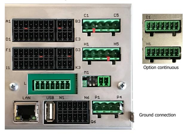
The Ground connection (flat plug 6,3mm) must be connected to an earth rail via a thick cable (>=4qmm) in the shortest possible way (<20cm)!
