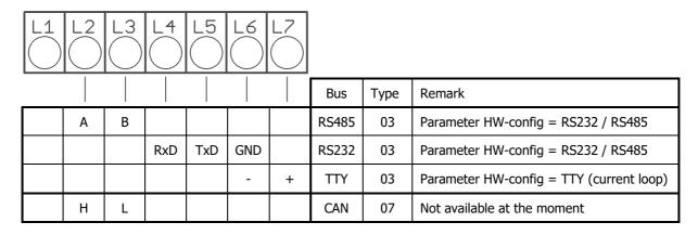
The serial fieldbus module (Type: 03) contains the three interfaces RS232, RS485 und TTY. By choosing the connection and setting the parameter "HW-config" the desired bus is selected.
