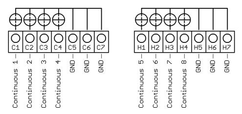
The GND connection terminals C5 - C7 and H5 - H7 are bridged. The output automatically switches to current or voltage, depending on the connected load.
