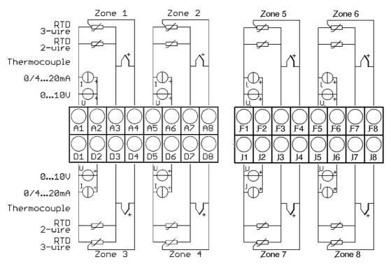
RTD/Ni120: The parameter "Sensor Settings / Sensor" has to be set accordingly to the connection diagram (2-wire/3-wire)
