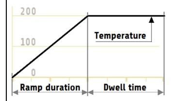
An exception is the ramp for the first step. Since the first step does not have a preliminary temperature, the ramp for all zones starts here with the current actual value of the first activated zone and ends at the temperature of step 1.
