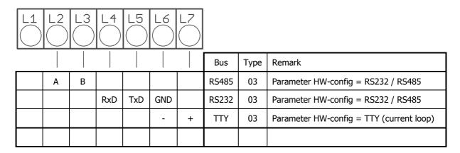
The serial fieldbus module contains the three interfaces RS232, RS485 und TTY. By choosing the connection and setting the parameter "HW-config" the requested bus is selected.
