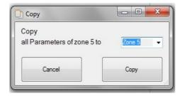
In this window, the selected zone can be copied to one or all zones of the same type. Same type zones are zones that are set via the parameter" sensor mix RTD/ TC" on the same type of sensor.
